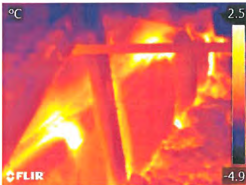
Image 16: Heat loss at top of boardroom wall
