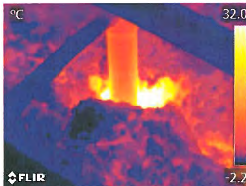
Image 13: Thermal image of an exhaust pipe
