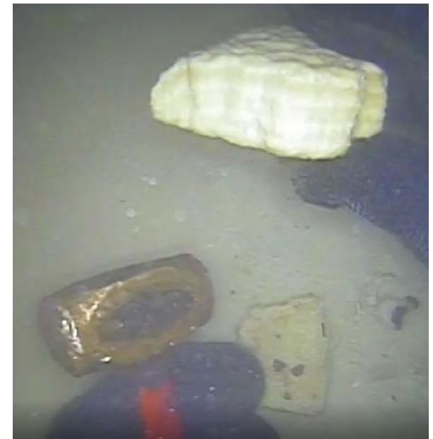
Precipitate found on the isolation valves in July 2020, with a sledgehammer for scale reference
