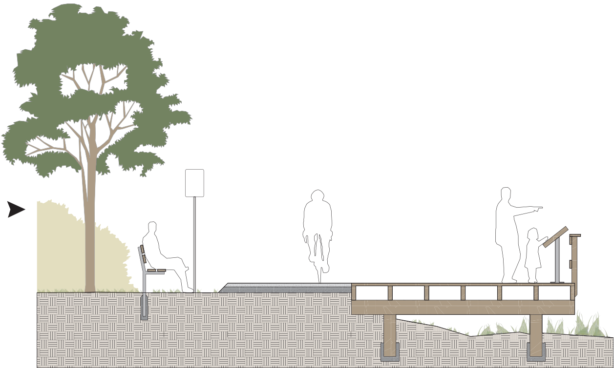
Trail Detail: Potential viewing platform over wetland/muskeg and rest area showing bench, signage and interpretive/information display.
