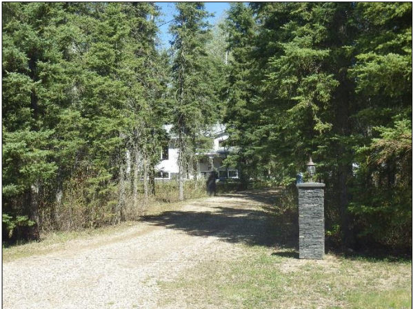
Inadequate Priority Zone 1 Clearance from Forest Fuels
