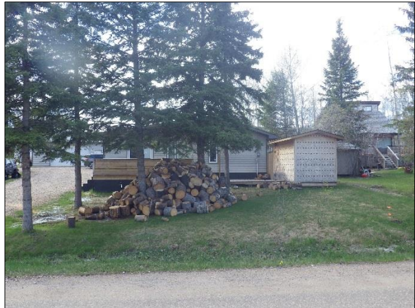
Inadequate Priority Zone 1 from Combustible Piles/Outbuildings
